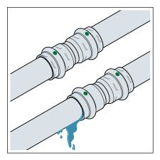
Viega press connectors are equipped with the SC-Contur. The SC-Contur is a safety technology that is certified by the DVGW and ensures that the press connector is guaranteed to be leaky in an unpressed state. In this way, inadvertently unpressed connections are noticed during a leakage test.
