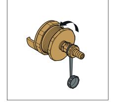
Insert the forcing plug in the connector.
