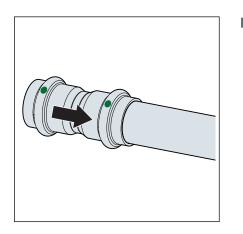
Push the press connector onto the pipe as far as it will go.
