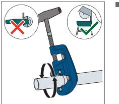
Cut the pipe using a pipe cutter or fine-toothed hacksaw. Avoid grooves on the pipe surface.
