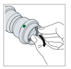
Do not use pointed or sharp-edged objects to remove the sealing element. They may damage the sealing element or the bead.
