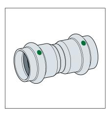
The press connectors have a circumferential bead in which the sealing element lies. The press connector is deformed upstream and downstream of the bead and permanently connected to the pipe during pressing. The sealing element is not deformed during pressing.
