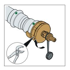
If a leak occurs while filling a system, retighten the forcing plug with a suitable tool.
